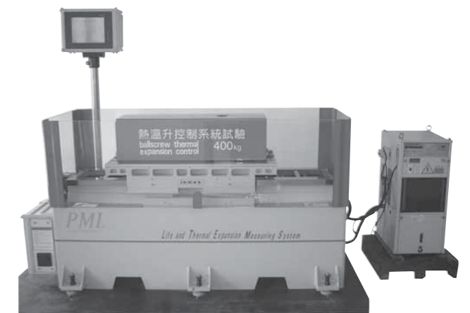
Fig.11.5 Thermal control system test unit
